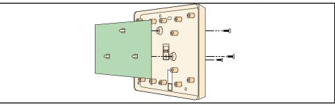
Install the cover tamper screw. Refer to illustration below.
