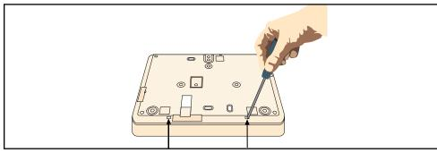
2. Use the mounting holes when installing to an elecrical box.
