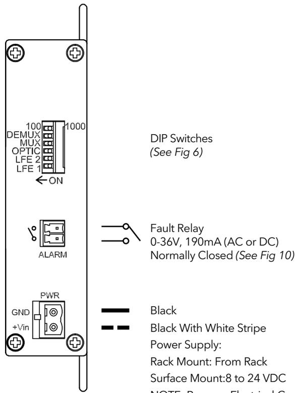
FIGURE 3 - Mini CNMC2+1SFP/M
