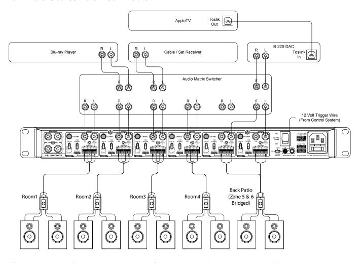
The diagram above illustrates the basic setup of a multi-room audio system with selectable source inputs routed through an audio matrix. See the notes below to understand the setup:
