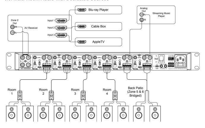
The diagram above illustrates the basic setup of a multi-room audio system with dedicated source inputs. See the notes below to understand the setup:
