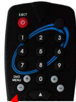
To bring up on screen menu select this key. Also the “Menu” key will work on most control systems.
