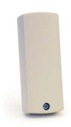
The Inovonics single input universal transmitter with wall tamper and EOL protection is designed for use with almost any standard contact or sensor. A 2.2K ohm end-of-line resistor is included with the transmitter and is required to operate it. The transmitter is fully supervised and includes a wall tamper switch that notifies the system when the transmitter is removed from its mounted surface.
