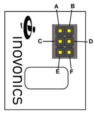
Figure 2 OEM connector pinout
