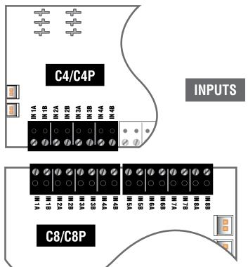
Each input on the C4 and C8 has an "A" terminal and a "B" terminal.
