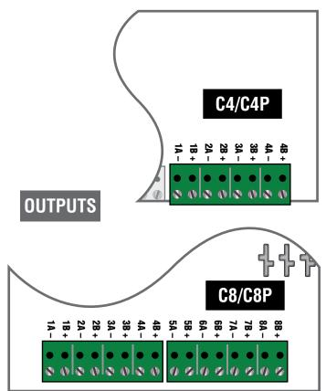
Each output on the **C4** and **C8** has an "**A**" terminal and a "**B**" terminal. The usage of these terminals varies based on the setting of jumpers **C** and **E** for the zone.
