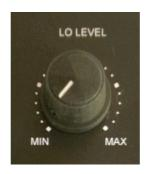
If the low level connection is to be made to left and right pre-amp outputs then a 12dB attenuator is available to balance the 0dB and +12dB phono inputs. See below.
