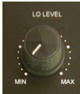
If the low level connection is to be made to left and right pre-amp outputs then a 12dB attenuator is available to balance the 0dB and +12dB phono inputs. See below.
