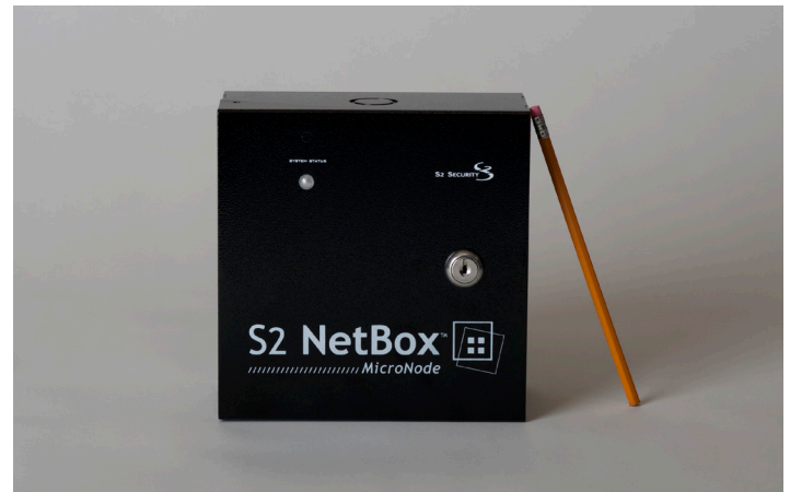
Small yet powerful: the S2 NetDoor controls two access points.
