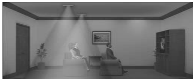
Conventional in-wall speakers used in ceiling applications allow coverage for only those listeners near the speakers.
